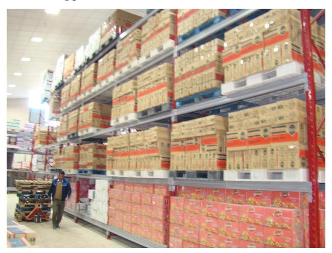
Pallet Rack heavy shelving with the name Arsa pallet rack is designed for preservation of pallet heavy loads. This type of shelving, using the maximum of warehouse height and design based on pallet dimensions, product dimensions, and product weight, causes the increase of significant volume in pallet maintenance.
