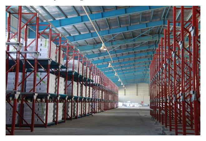
Drive-in system is a self-drive system which is suitable for maintenance of heavy items by special machines (forklift, reach truck, and stacker) for loads of same kind.
